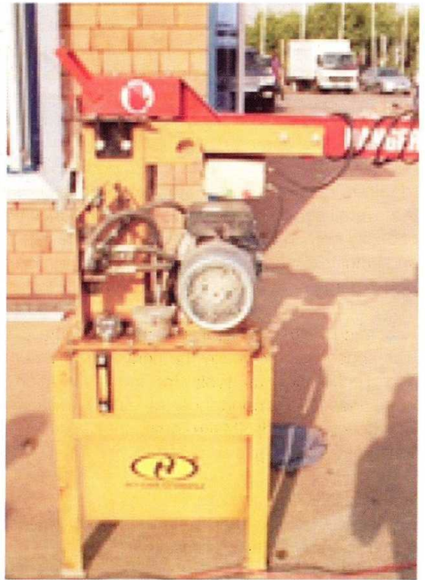
The NBRI Hydrafoam Interlocking block making machine
