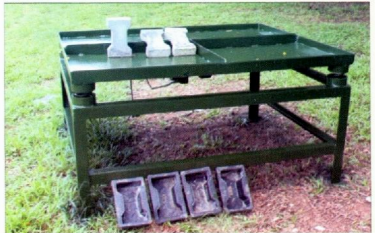
NBRRI VIBRATING TABLE (MACHINE) Picture shows the Vibrating Table, Plastic Moulds and Paving Stones produced
