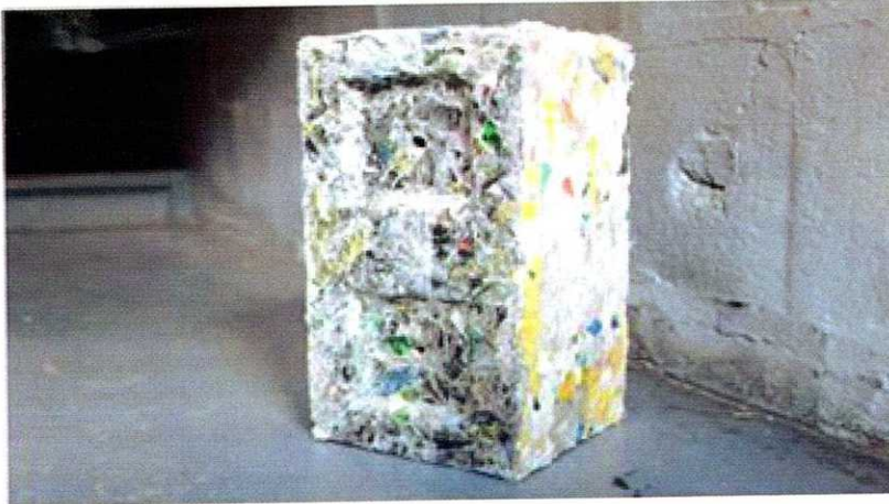
Figure 8: Plastic Bricks made from used Water Bottles
