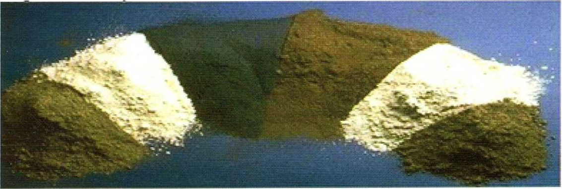
Figure 13: Green Substitutes to Cement known as supplementary cementitious materials (From the left to the right, class C fly ash, metakaolin (calcined clay), silica fume, class F fly ash, ground granulated blast furnace slag, and calcined shale)
