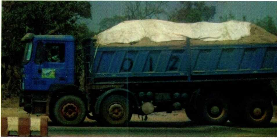
Plate 9: Typical 4-Axle truck loaded with sand
