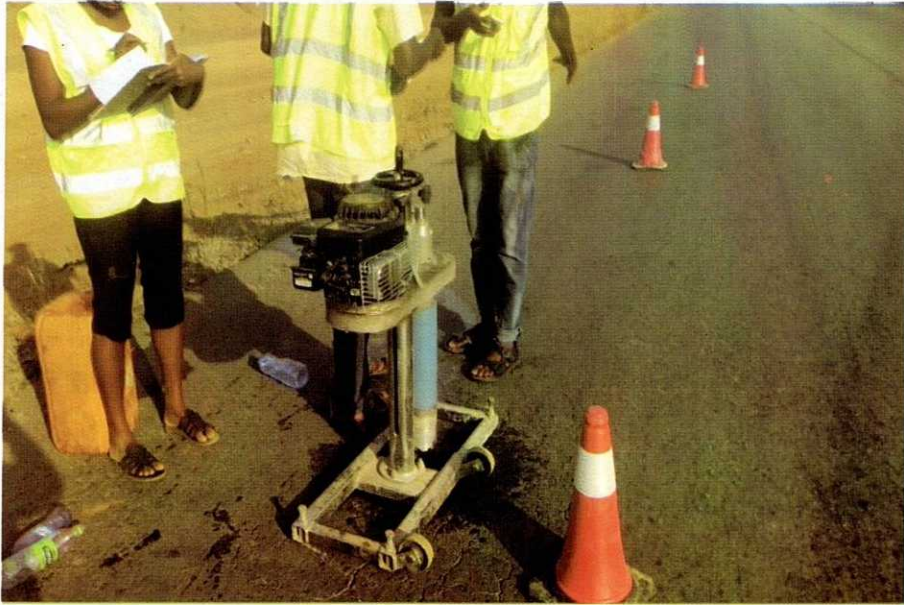
Plate 5: COLLECTION OF CORED SAMPLES FROM THE SITE.
