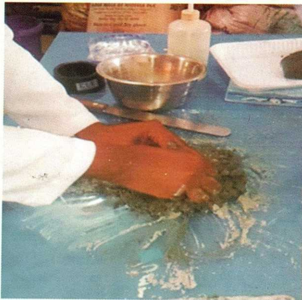
Mixing of cement paste
