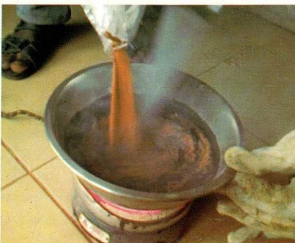
Mixing of plastic/bitumen mix with laterite
