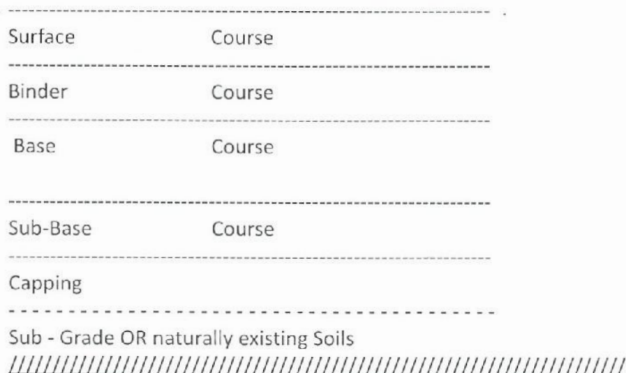
Figure 2: Flexible Road Structure typical cross-section
