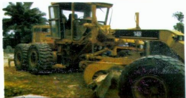
Photo 39 – A grader that is also typically used to scarify and grade road pavement
