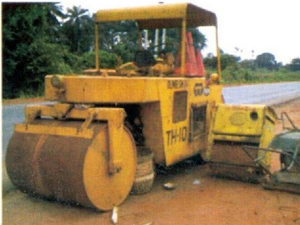
Photo 40 – A steel drum roller and a smaller hand-operated vibratory compactor
