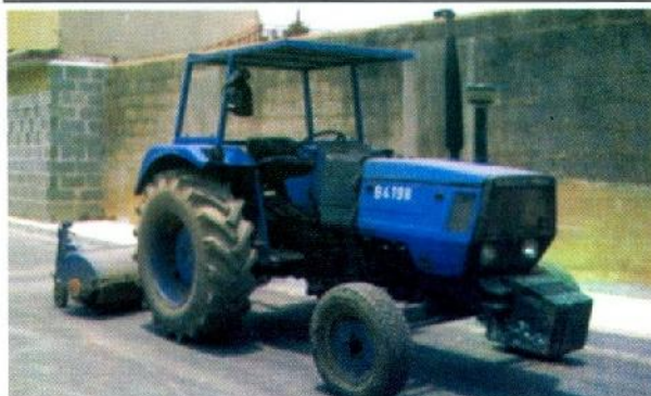
Photo 9 – A mechanical sweeper for cleaning pavement surface prior to tack coat application
