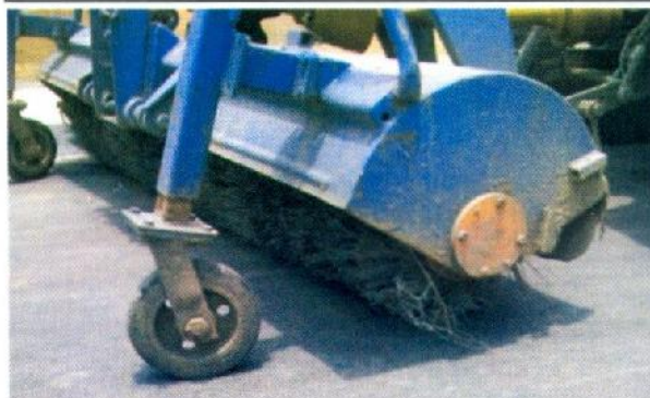
Photo 10 – Close-up view of the iron strands of the mechanical sweeper (Courtesy: Julius Berger Nig. Ltd.)
