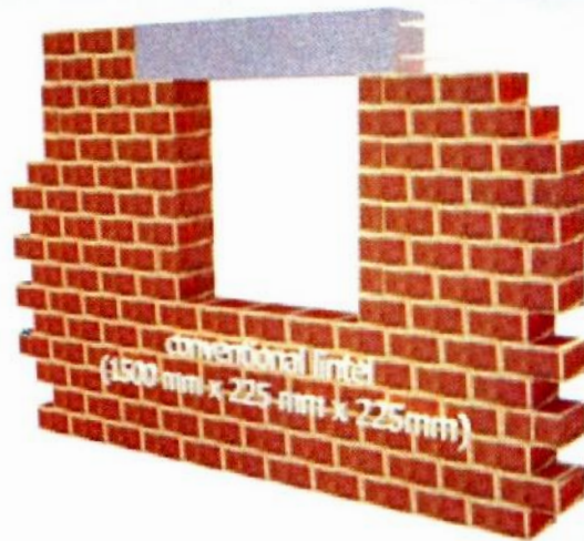
Figure 12: Conventional lintel measuring 1500mm X 225mm X225mm
